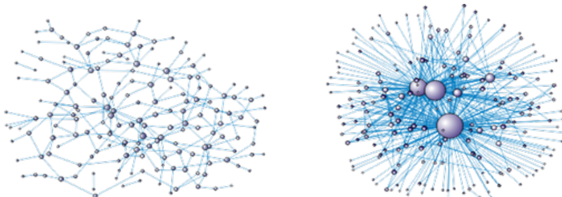
Figure 4. Distribution of vertex degrees. Figure showing two networks with the same number of vertices and connections, but with different degree distribution. Source: http://www.if.pw.edu.pl/~agatka/moodle/charakterystyki.html
