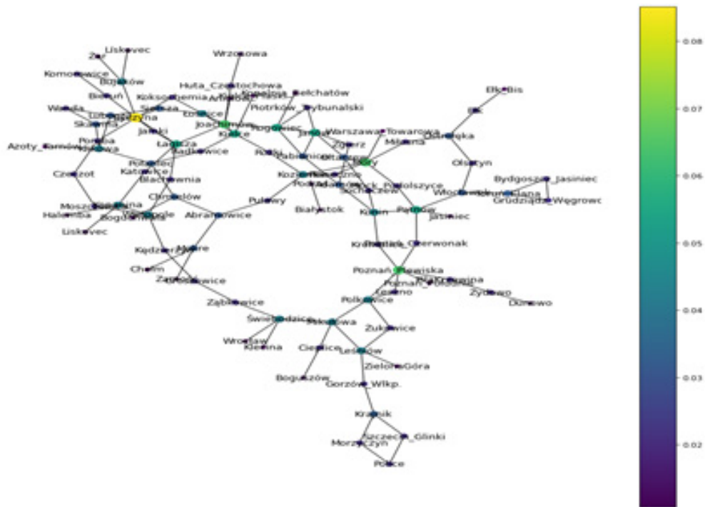
Figure 1. 220kV network graph with degree centrality. Source: the authors' research.
